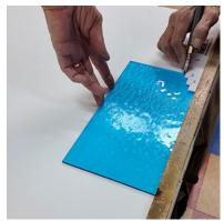
Press glass firmly with left hand up against pre-attached straight edge. Place cutter firmly in appropriate measured slot (example 1" shown). Run Ultimate Strip Guide and cutter along straight edge.
