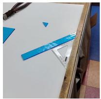
Snap off and dispose of this set up piece. Place the strip against an angle guide again and use guide at same measure slot as the strip size you cut originally (example 1" shown).
