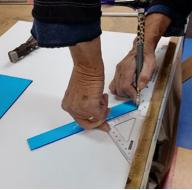
Snap off strip. Place strip along an angle guide and use the strip guide to cut off 90 degree edge to make it appropriate angle for diamond. (You can use any slot on the strip guide for this purpose)
